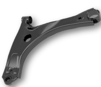
Existing steel component 4.4kg
