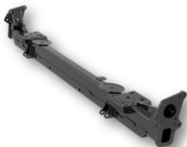
Existing steel component 39.75kg
