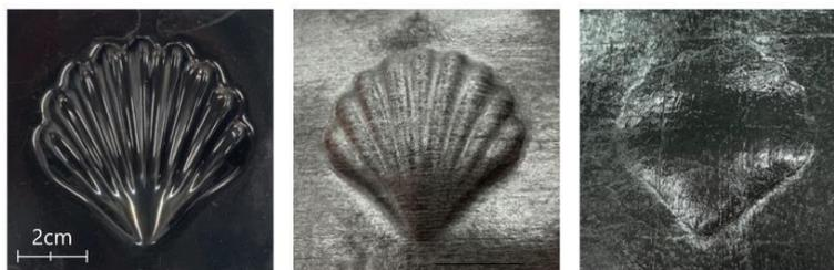
Figure 2: Shell mould (left) and formed preforms; aligned fibre (centre) and continuous fibre (right).
