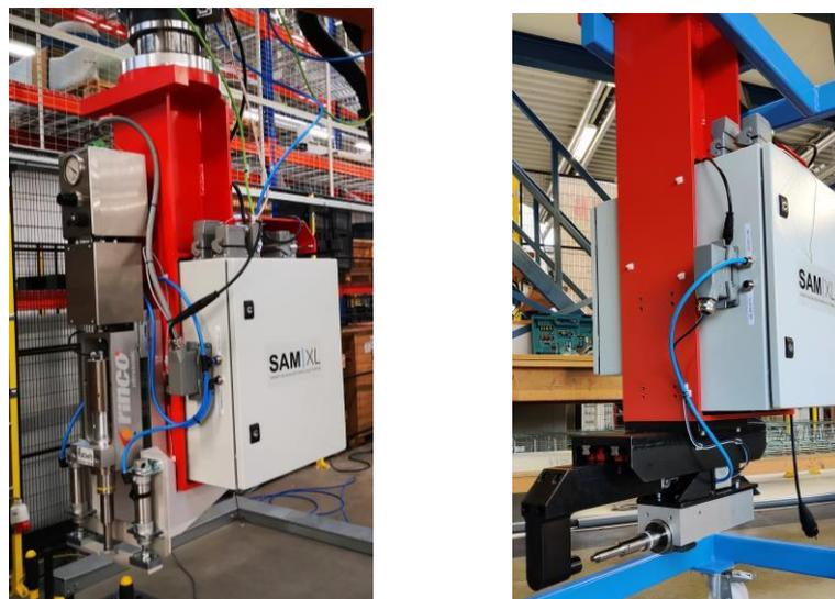
**Figure 2: Robotic End-Effector for Clip-To-Skin (left) and Clip-To-Frame (right) Ultrasonic Welding**
