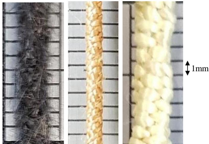
Figure 3: Circular cross section carbon fibre-epoxy rods overbraided with Toray T300 carbon (left), Teijin high modulus Zylon (centre) and Teijin Twaron 2200 aramid (right).
