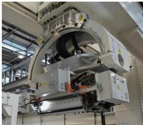
Figure 3. A 1.3 m FibreROLL system, gantry mounted
