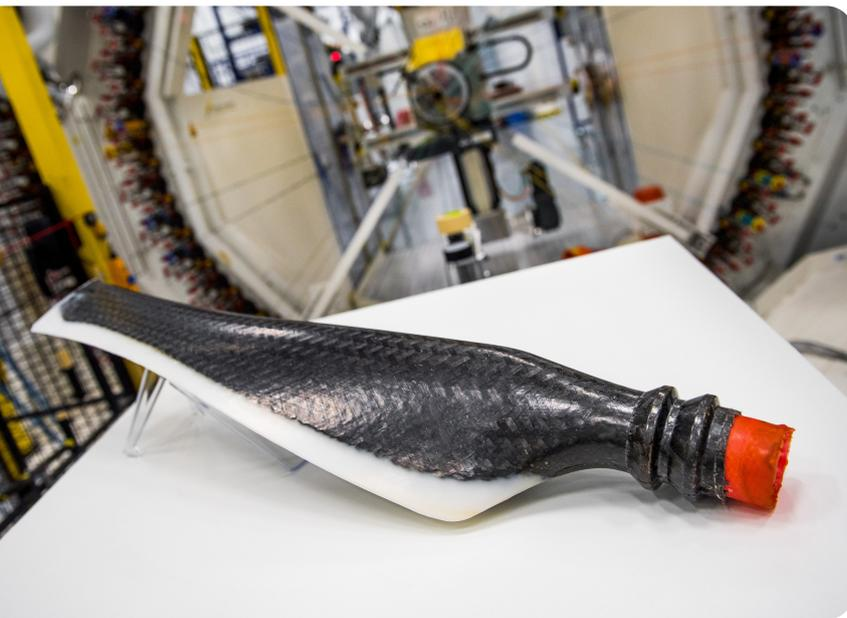
Dowty Propellers, part of GE Aviation, approached the NCC to join an exciting collaborative programme to design and develop composite propeller blades that not only reduce costs but improve performance. This innovative work would accelerate Dowty's digital manufacturing capabilities, demonstrating the UK's world-leading expertise in propulsion technology for turboprop aircraft.
