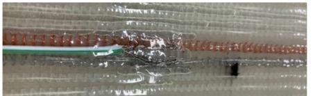
Novel solution: A post-fusion and demoulded panel showing interwoven connections within the glass fibre material that are capable of detecting accurate temperature variations.
