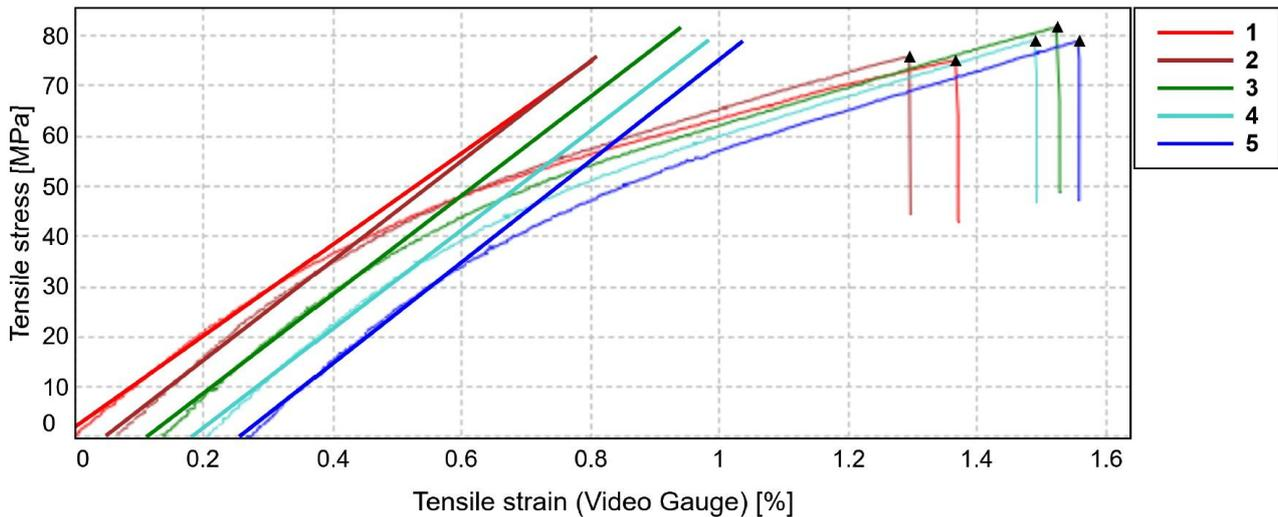
This graph shows tensile testing results of Lincore coupons indicated a tensile strength of 78.2 MPa and Young's Modulus of 9.77GPa
