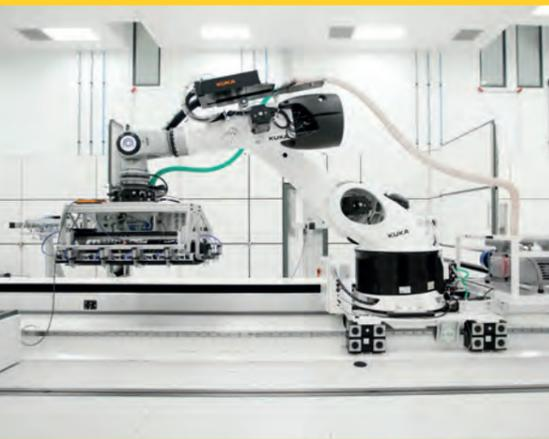
The NCC Smart Factory Innovation Hub Test Bed provides access to a virtual and physical test bed environment that concentrates on the Automated Preforming Cell (APC), a state-of-the-art facility for automation of the preforming process of composite component manufacture. It is specifically focused on the manipulation, forming and consolidation operations related to the preforming of dry fibre.
