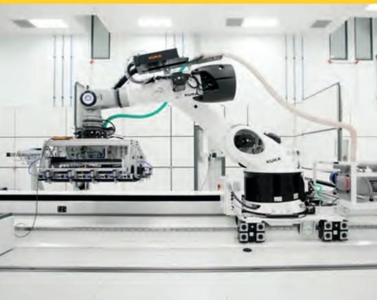
The NCC Smart Factory Innovation Hub Test Bed provides access to a virtual and physical test bed environment that concentrates on the Automated Preforming Cell (APC), a state-of-the-art facility for automation of the preforming process of composite component manufacture. It is specifically focused on the manipulation, forming and consolidation operations related to the preforming of dry fibre.
