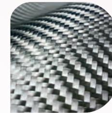
Composite material strength lies in the uniform pattern of either unidirectional or interwoven carbon fibres lying undisturbed
