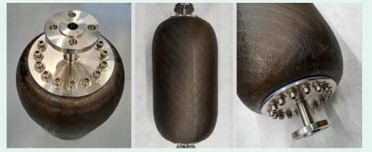
The 30-litre tanks were designed for a pressure of 8 bar and manufactured onsite using automated fibre placement.
