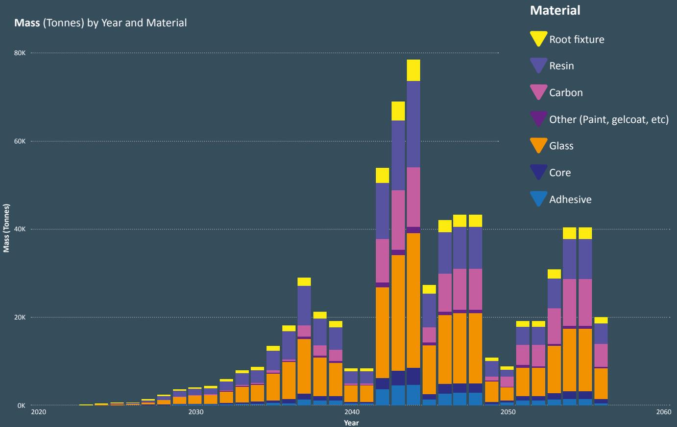
Figure 4 Offshore blade masses by material
